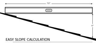
Set one end of a 12" level on the roof surface – make it level.
