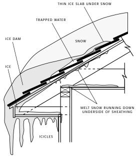
"...CONTINUALLY THAWING AND REFREEZING OF MELTING SNOW FORM ICE DAMS."
