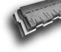
The coating section comes next where the asphalt combined with a stabilizer is added the top and bottom of the saturated felt sheet.
